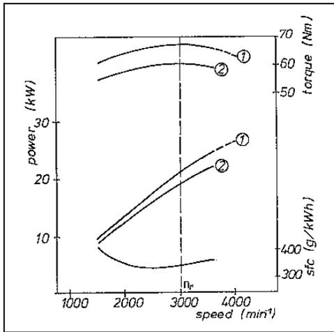
Fig. 7.6: Typical engine performance curves showing the power, torque and specific fuel consumption as a function of the speed. 1 maximum shortterm performance, 2 allowable performance for continuous operation.
