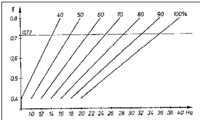
Fig. 4.2: Calorific value of biogas as a function of the density and volume %-age of its CH<sub>4</sub> content ( $\rho=0.72$  is the density at a standard condition)
