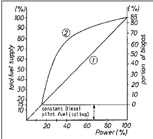
Fig. 5.9: Fuel supply vs. power output Diesel pilot fuel constant, biogas controlled (manually or automatically) according to power demand. 1 total fuel, 2 portion of biogas in total fuel (simplifying assumption: sfc=constant).
