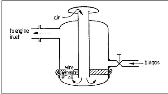
Fig. 5.3: Air filter modified into mixing chamber
