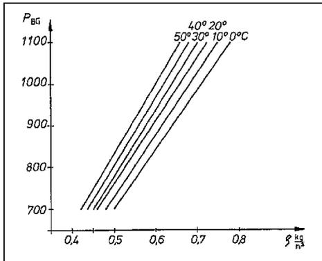
Fig. 4.1: Density  $\rho$  of CH<sub>4</sub> as a function of biogas pressure and temperature
