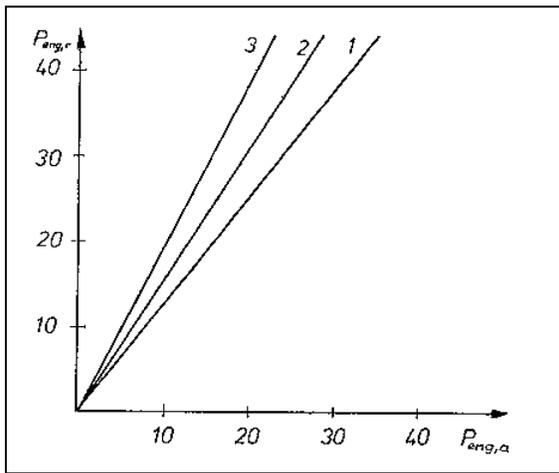
Fig. 7.8: Relation of rated power of engine (before modification),  $P_{eng,r}$  and its actual power output  $P_{eng,a}$  at optimal economic conditions with biogas. Operational speed = 0.8 X max. speed. 1 diesel gas (dual fuel) engine operating short periods only, 2 as 1 but operating continuously, 3 Otto biogas engine, continuous operation.
