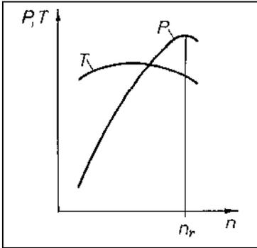
Fig. 3.2: Engine power output P and torque T as a function of engine speed n:  $n_r$  marks the rated speed.
