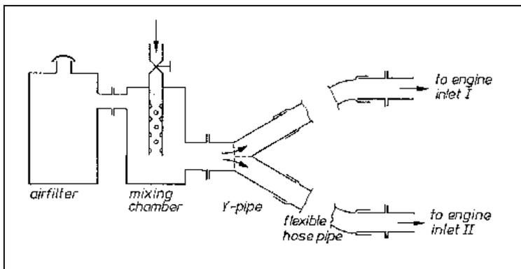
Fig.5.7: Mixing chamber connected to a V-type engine (engine)
