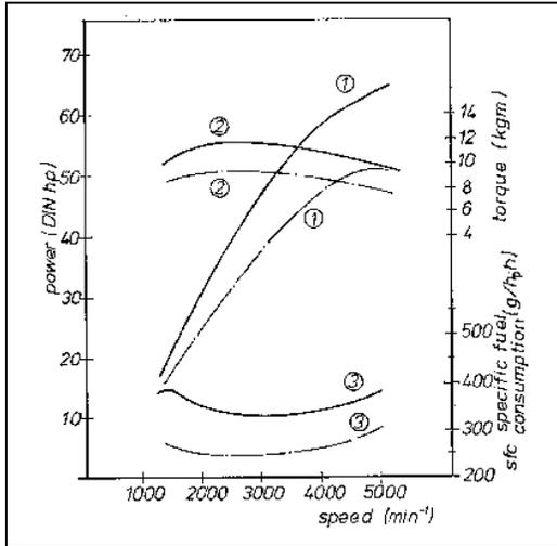
Fig. 6.1: Performance diagram of an Otto engine using liquid fuel (—) and methane(---) alternatively (Rodagas).
