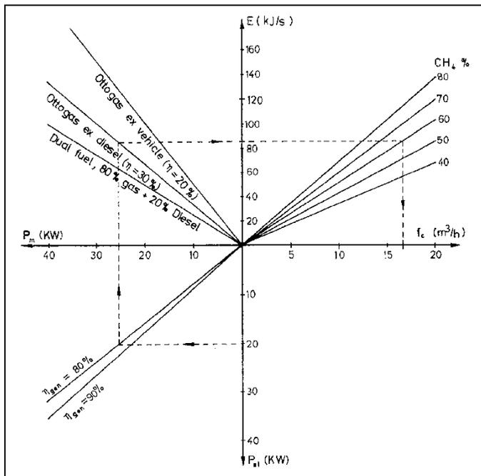
Fig. 7.9: Nomogram for the relation of fuel consumption/fuel demand  $f_c$ , biogas quality  $CH_4\%$ , fuel energy flow  $E$ , type of engine used, mechanical power output  $P_m$ , electric generator efficiency  $\eta_{gen}$ , and electric power output  $P_{el}$ . Basic gas data assumed: temperature 25 °C, pressure 960 mbar, ref. humidity 100%.
