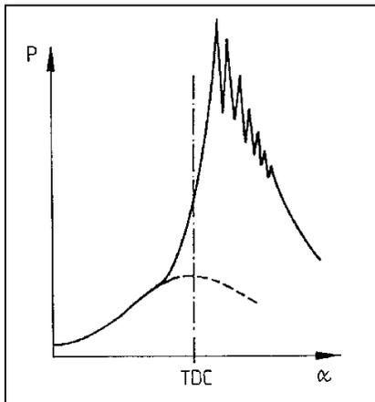
Fig.4.4: "Knocking" in a p, alpha-diagram of an engine
