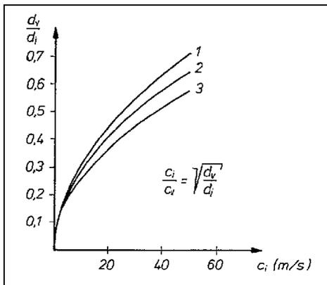
Fig. 6.5: Venturi diameter ratio  $d_v/d_i$  as a function of intake velocity  $c_i$  and the required velocity at the venturi bottleneck  $c_v$
