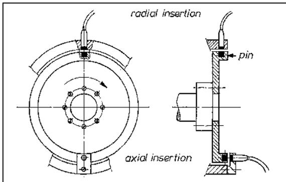
Fig. 5.14: Fixing the pick-up in the casing and the flywheel, two different versions; upper half: radial insertion, lower half: axial insertion.
