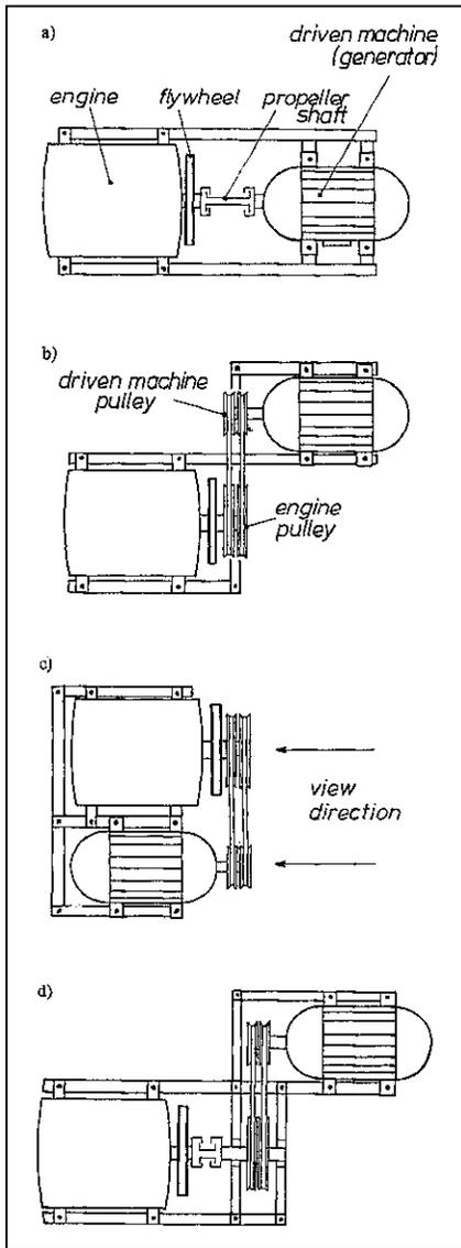
Fig 7.10: Alternative positioning of engine and driven machine depending on direction of rotation and type of transmission. Direction of rotation is given as viewed facing the shaft ends, example c).
