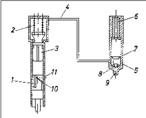
Fig.3.10: Principal scheme of injection system (numbers correspond to text).
