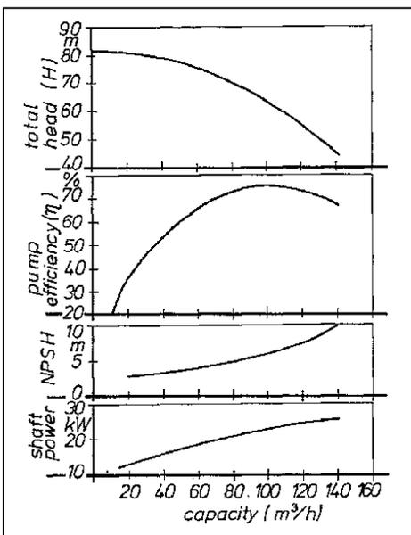
Fig. 7.12: Characteristic curves of a radial centrifugal pump at constant speed (KSB)
