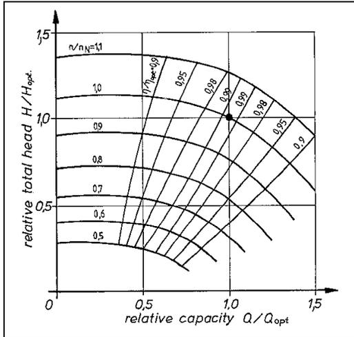
Fig. 7.13: Performance chart of a speed-controlled centrifugal pump (KSB)
