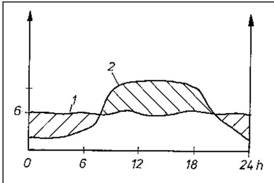
Fig 24: Daily profiles: 1 biogas and potential power production, 2 power demand; option for storage of excess biogas for periods of biogas shortage. /// excess biogas production \\biogas shortage
