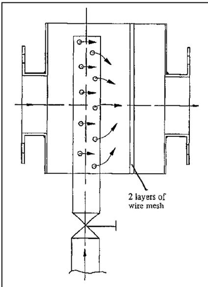
Fig. 5.5: Mixing chamber with gas distribution pipe and wire mesh for intensive mixing
