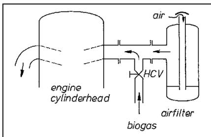
Fig. 5.6: T-joint mixer installed between air filter and engine inlet
