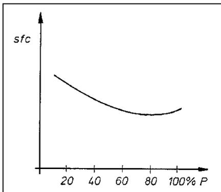
Fig. 7 7: Specific fuel consumption, sfc, as a function of power output at constant speed (schematic)
