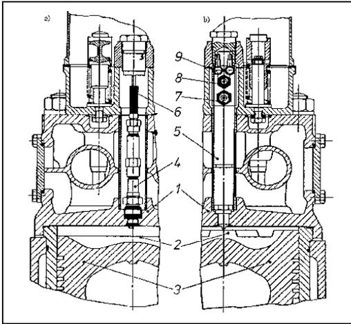
Fig. 5.16: Cylinder head modified with spark plug on increased combustion chamber volume (a) vs. original diesel version with injector (b)
