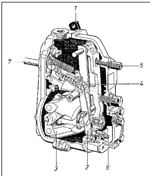
Fig. 5.8: Governor for diesel fuel injector pump (Bosch).
