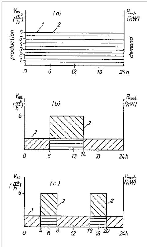
Fig. 7.5: Daily production and demand profiles for the example. - biogas production directly consumed. /// excess biogas production for storage, \\\biogas drawn from store to cover for actual shortage.
