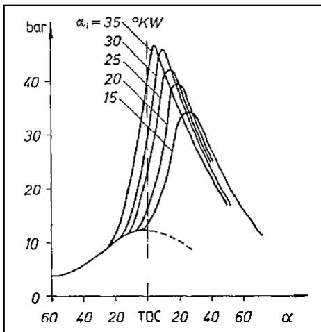
Fig. 3.5: Course of pressure as a function of the crank angle  $\alpha$  (point) of ignition  $\alpha_i$
