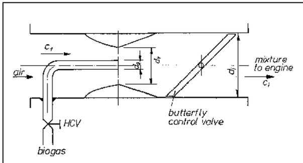
Fig. 6.3: Venturi mixer with a single gas inlet nozzle.
