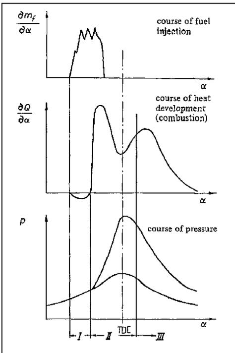
Fig. 3.9: Courses of fuel injection, combustion and pressure as a function of the crank angle  $\alpha$
