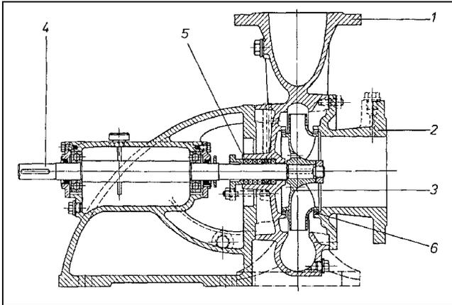
Fig. 7.11: Cross-sectional view of single-stage centrifugal pump (KSB).
