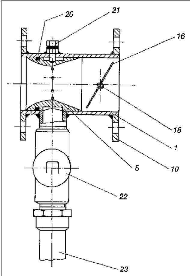
Fig. 3: Venturi mixer assembly
