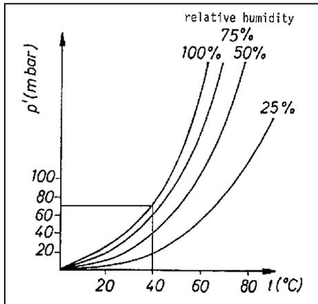
Fig. 4.3: Partial pressure of water vapor in a mixture with biogas as a function of a biogas temperature and relative humidity
