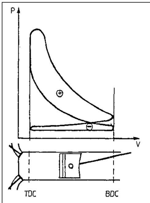
Fig. 3.3: Pressure, volume (p, v) diagram of a 4-stroke engine cycle
