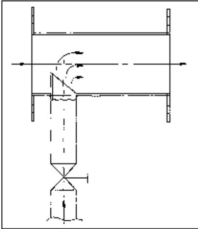
Fig. 5.4: T-joint mixer with oblique, protruding gas inlet
