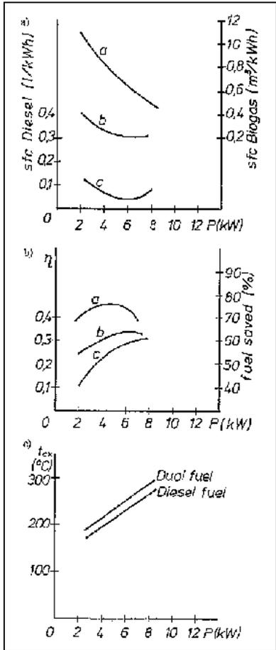
Fig. 5.12: Performance charts of a 10 kW single cylinder gas engine with biogas at  $n=1500 \text{ min}^{-1}$  (from[11]).
