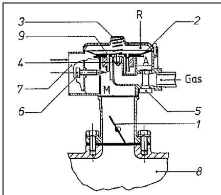
Fig. 6.6: Cross-sectional view of gas mixing valve.
