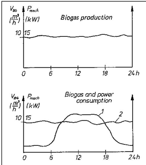
Fig. 7.1: Fuel and power production vs. consumption/demand profile. 1 typical example for operation of machines during the day and little lighting at night, 2 demand balanced and adapted to biogas production.
