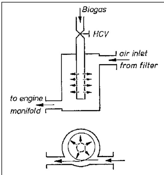
Fig.5.2: Simple mixing chamber with hand - controlled valve (HCV)
