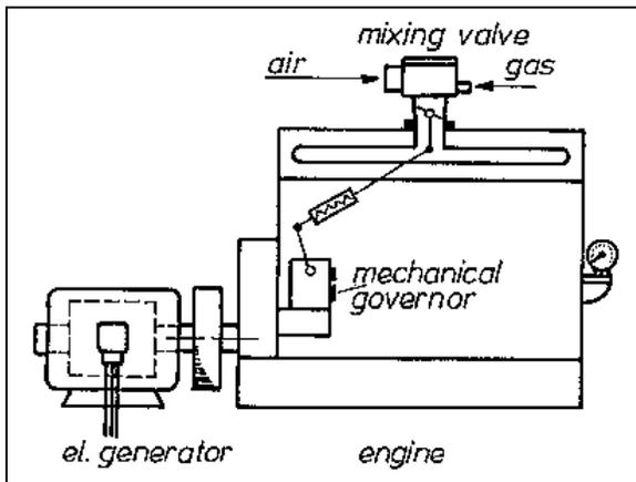
Fig. 6.8: Mechanical speed governor directly acting on the butterfly throttle in the mixing valve.
